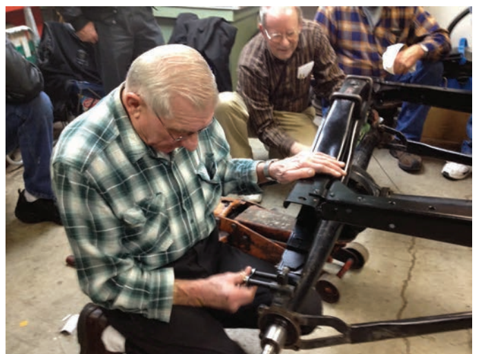
Club members used a floor jack to lift the rear axle in place while installing the rear spring shackles.
