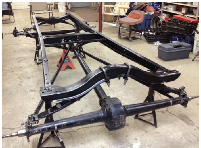
By the end of the evening the Model A chassis looked like this, with springs and axles in place.
