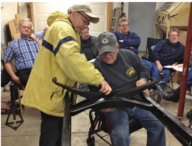
Scott Tilton, left, and Roger Olsen test fit the front spring into the Model A frame.
