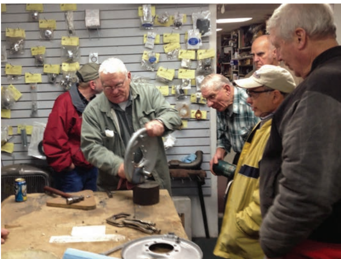
Al Downs used both a grinder and a torch while preparing the old backing plates for reuse on the chassis.
