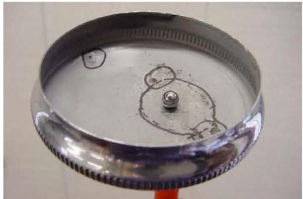
On a roll now, I was able to push up all the dents, file the cap to reveal other low spots, sand with 320, 400 and 600 wet-or-dry paper and polish. I painted the inner cap with anti-rust silver and pressed it back into the outer using some Loctite blue medium strength.
