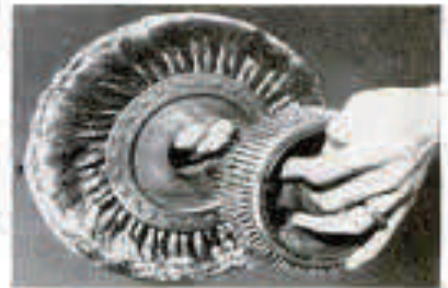
1 OLD RUBBER COMES OFF The first step in rebuilding a worn-out tire. With a long, sharp knife made of file steel, a workman pares off the old rubber in strips, going as close to the cord as he can with safety.
