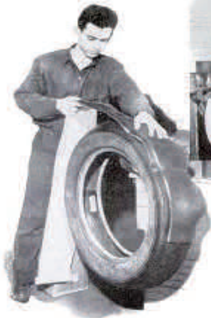
3 NEW TREAD STOCK APPLIED TO CORD The body of the tire is given two coats of rubber cement, as shown in the small picture. Then new tread stock like that used in new tires is applied to cover the top and sides.
