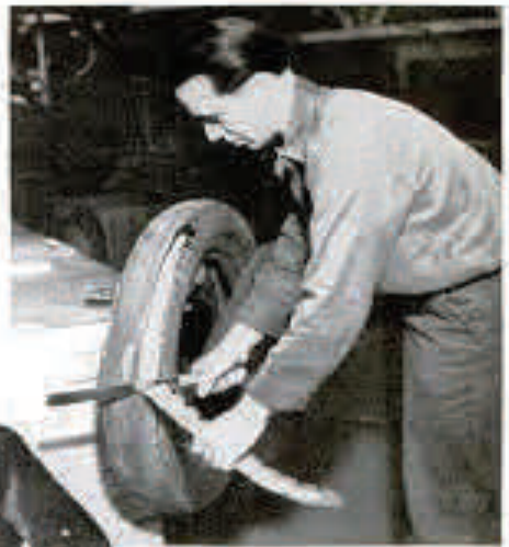
1 OLD RUBBER COMES OFF The first step in rebuilding a worn-out tire. With a long, sharp knife made of file steel, a workman pares off the old rubber in strips, going as close to the cord as he can with safety.
