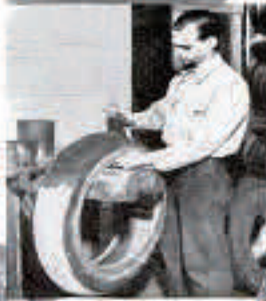
2 Rubber is buffed off the shoulders with a tach-studded band, and the cushion under the tread is ground off with a steel brush. The photo at right shows the band and brush.
