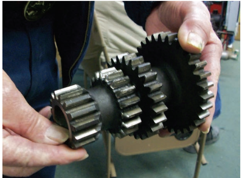
Right: The gear cluster is the heart of our Model A transmissions.
