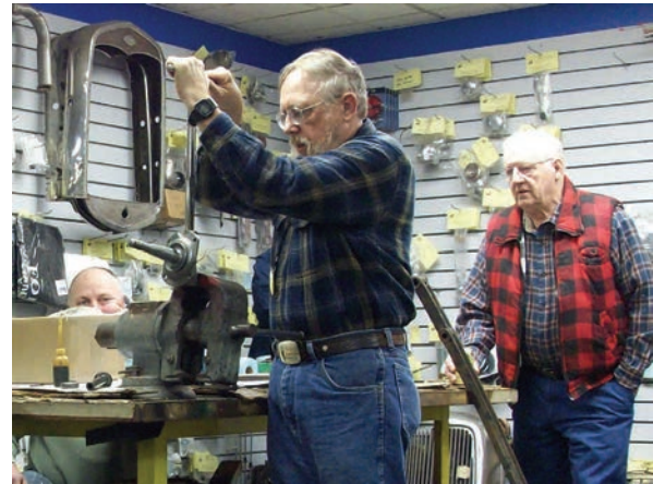
Bob twists the reaming tool through the bushings. The tool cuts tiny slivers from the inside of the bushings to bring them into alignment.
