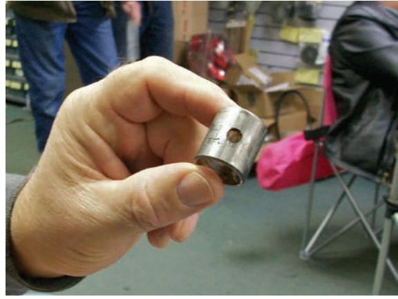
Here is one of the bushings before it was inserted into the spindle. The hole on the side matches up with a grease fitting on the spindle.
