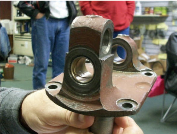
Here is the spindle with its two shiny new bushings press fit into the assembly.
