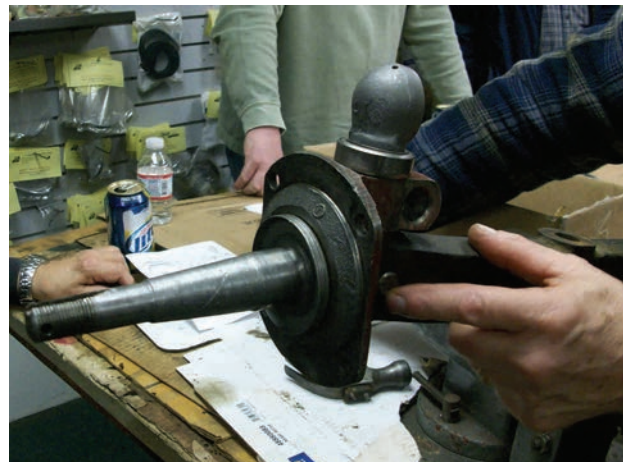
Here's a close look at the king pin, with its ball-shaped head, holding the spindle onto the end of a Model A axle.
