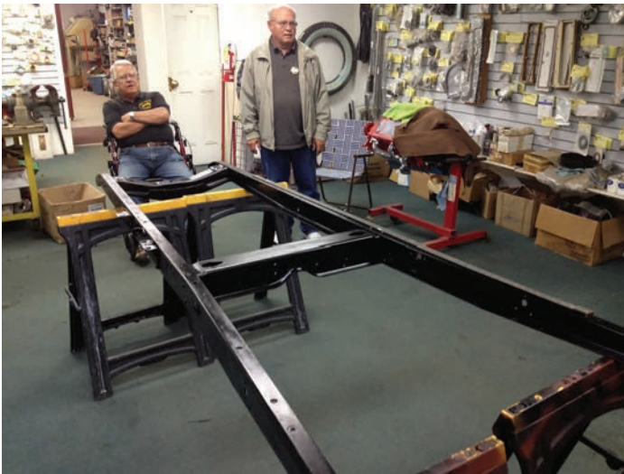
The starting point was a bare Model A frame that had been cleaned up and spray painted black.
