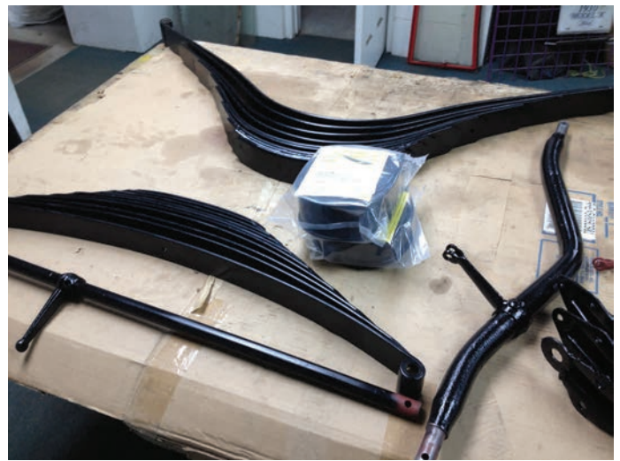
Club members at the tech meet installed a brake cross shaft and anti-squeak liners between the leaves of the front and rear springs.
