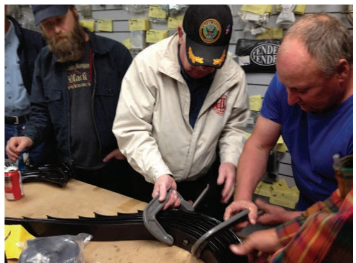
Once the padding was in place between leaves of the spring, Gary Schwabe used a C-clamp to hold the assembly together.
