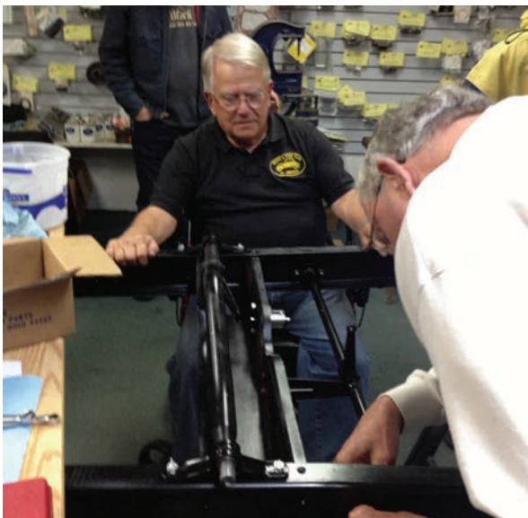
Roger Olsen watches as club members install bearings for the brake cross shaft into the newly painted frame.
