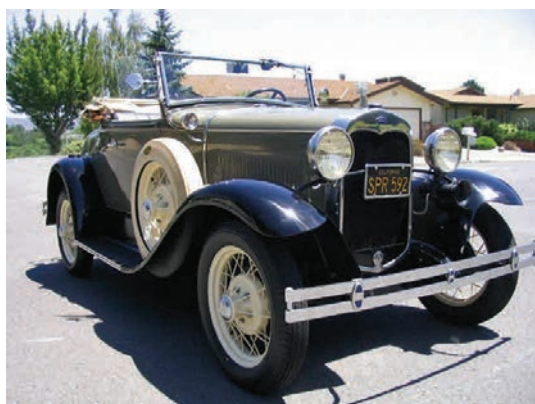
1930 Model A's are easier to identify: taller, stainless-steel radiator shells with a blue Ford oval emblem at the top.
