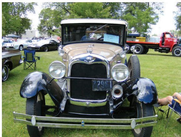
1928 and 1929 Model A's had shorter, nickel-plated radiator shells and bends at the ends of the bumpers. This is a 1929.
