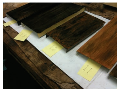
Different amounts of graining paint created different effects and can be used to imitate different types of wood.
