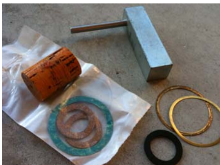
Gas gauge parts such as cork floats and various gaskets are available from parts stores, as well as the specialized gas gauge removal tools.
