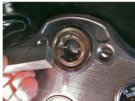
The metal-block tool is designed to fit into the star-shaped opening in the gas gauge. Twist the block to remove the inner portion of the gauge.
