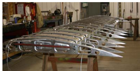
Above: Wing being assembled
