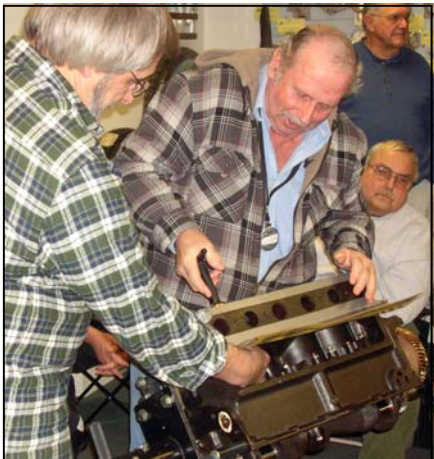
Tony instructing Ron how to hand grind valve seats to the proper degree easily by hand.
