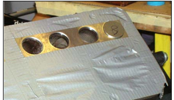
See the neat well done hand grinding job on the valve seats by our Model A volunteers? Notice "#8" on a valve? Each valve is fitted individually. Notice also how the block is sealed off so that shavings will not fall in any ports. This makes it easier to clean out the block.
