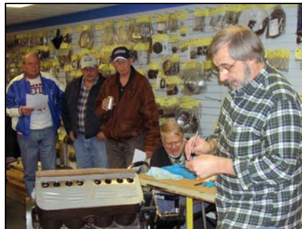
Jim, Dennis, and Jim paying close attention to Tony instructing us how to properly grind valve seats.
