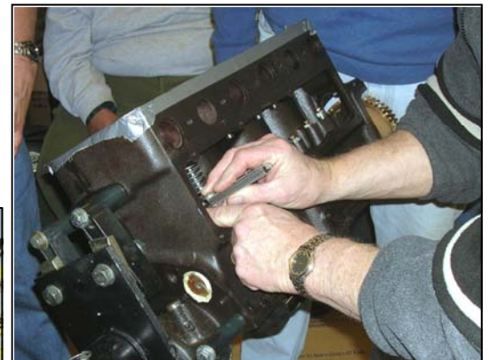
Tony adjusting the clearance with the feeler gauge on the adjustable valve lifters. He will set the correct gap on the lifter.
