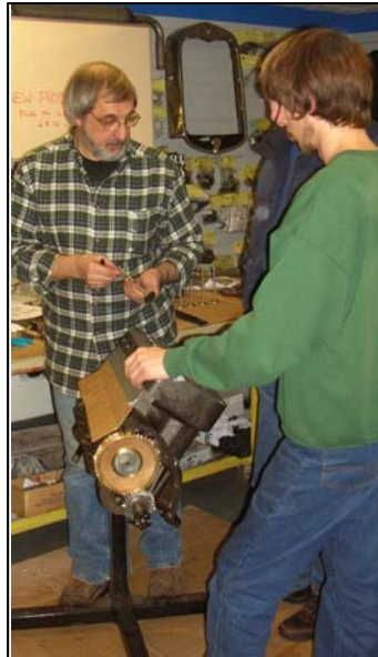
Tony showing the new type valve to Aaryn which will be installed in this motor. This is after all valve seats have had the shavings cleaned out.
