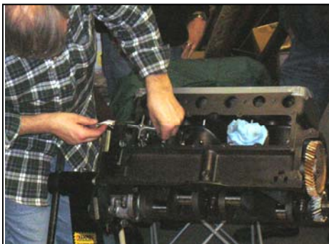
Tony installing the valve. Notice how the valve spring is compressed so he can install keepers to hold the valve spring in place.
