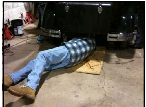
Installing seat belts in this Model A during January's technical meet included getting beneath the car to anchor the belts to the frame.
