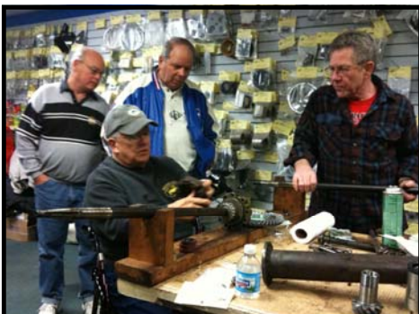
During February's technical meet, club members learned how to rebuild a Model A rear end, including the driveshaft and axle.
